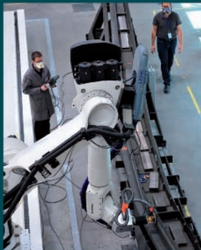
One of the IRT's research project : Robofin about a new robotic solution to finish large size parts
