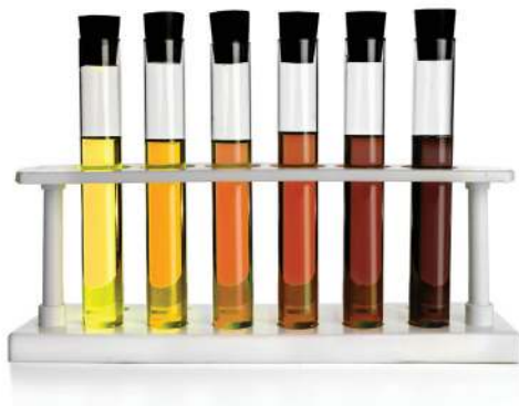
Sebelum ada ConSite Oil, mekanik menganalisis kondisi oli berdasarkan warna. Before ConSite Oil, mechanics analyze oil condition based on color
