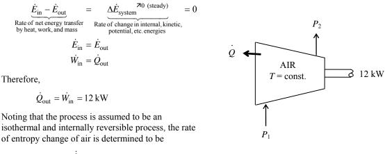
$$\Delta \dot{S}_{air} = -\frac{Q_{out,air}}{T_{sys}} = -\frac{12 \text{ kW}}{298 \text{ K}} = -0.0403 \text{ kW/K}$$
