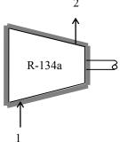
There is only one inlet and one exit, and thus  $\dot{m}_1 = \dot{m}_2 = \dot{m}$ . We take the compressor as the system, which is a control volume since mass crosses the boundary. The energy balance for this steady-flow system can be expressed in the rate form as
