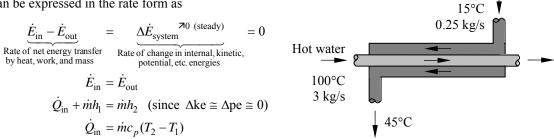
Then the rate of heat transfer to the cold water in this heat exchanger becomes
