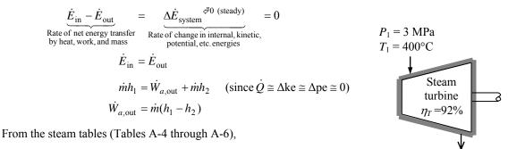
$$P_{1} = 3 \text{ MPa} \begin{cases} h_{1} = 3231.7 \text{ kJ/kg} \\ s_{1} = 400^{\circ}\text{C} \end{cases} P_{2} = 30 \text{ kPa} \\ s_{2s} = 30 \text{ kPa} \\ s_{2s} = s_{1} \end{cases} \begin{cases} x_{2s} = \frac{s_{2s} - s_{f}}{s_{fg}} = \frac{6.9235 - 0.9441}{6.8234} = 0.8763 \\ h_{2s} = h_{f} + x_{2s}h_{fg} = 289.27 + (0.8763)(2335.3) = 2335.7 \text{ kJ/kg} \end{cases}$$
