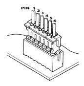
Sensored type compatible speed controls must use the six position JST header part number X-6B-ZRSMX-TK (where X denotes the style of the header) or equivalent. The power motor wire connections must be clearly marked A, B, C on both speed control and motor. A for phase A; B for phase B; C for phase C
