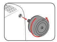
2 Remove the screw at the top of the filter.
