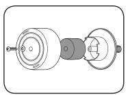
4 Reassemble the filter and then fit to the air compressor.
