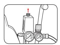
2 Switch off the mains power supply and remove the electrical plug.
