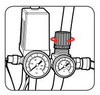
**Note:** Air must be flowing through the quick release air outlet, and the attached air tool in order to obtain the correct output reading on the pressure gauge.
