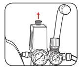
3 To switch the compressor off, push the on/off switch down into the off position.
