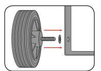
2 From the inside of the wheel bracket, place a washer and spring washer on the wheel bolt. Fasten the wheel bolt in position with a nut.
