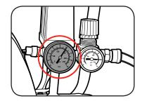
**Note:** When the maximum preset tank pressure is reached, the motor will automatically switch Off. As the compressed air is used, the pressure will drop until it reaches the preset minimum pressure, when the minimum pressure is reached the compressor will turn on again automatically to build up/maintain pressure.
