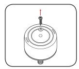
3 Open the filter and carefully clean by tapping or blowing it with low pressure compressed air (approx. 3 bar).
