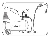
2 To switch the compressor on, pull the on/off switch up into the on position.
