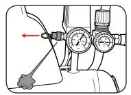
3 When the ring on the safety valve is released the air discharge should stop.
