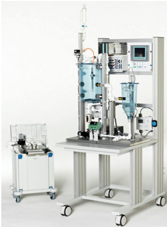
Picture of the Wastewater Treatment System
