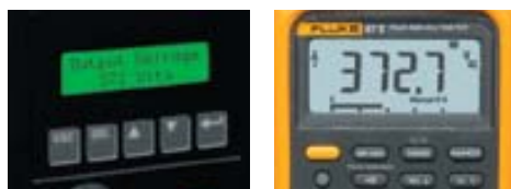
Figure 3. Output voltage reading with low pass filter enabled.
