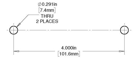
Nitro HD Joystick – (Panel top mounting, with enclosure)
