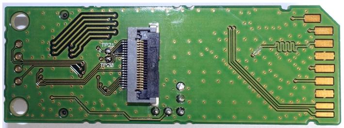
Refer to **Figure 9**: **Murata i.MX InterConnect Adapter V2 Adapter - Bottom**. Both TP20 and TP21 short pads are closed to connect WL\_REG\_ON and WL\_HOST\_WAKE respectively. WL\_HOST\_WAKE is an optional out-of-band interrupt signal that is not defined in this Quick Start document. It will be documented (and optionally enabled) in future version. For additional specific information on default configuration, please reference the Murata Hardware User Manual.
