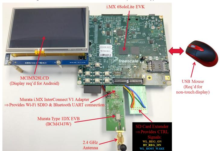
Figure 3: i.MX 6SoloLite EVK with V1 Adapter and Type 1DX EVB
