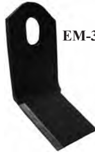
EM-217-1 Heavy-Duty Blade (.25" Thick) 1.8" Wide, 3.6 Tall, .25" Thick, 1.2" x .58" Mtg. hole
