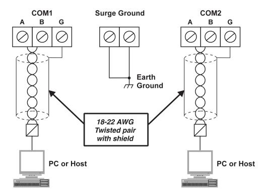
Figure 3-4: RS-485 Communications Connections
