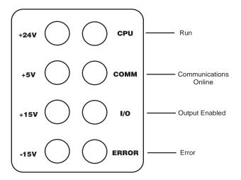
Figure 11-1: 8130 RTU LED Indicators
