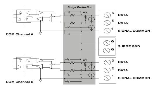
Figure 5-5: Model 8203 COM Channels Schematic
