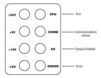
Figure 11-2: 8130 RTU LED Indicators under Abnormal Conditions
