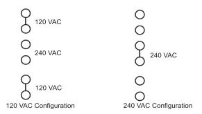
Figure 4-6: 120/240 VAC Configurations
