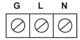
Figure 4-5: AC Input Terminal Block
