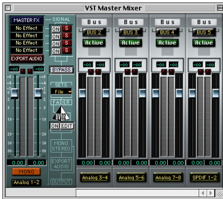
Figure 8-4: Use the output buttons at the bottom of each channel strip to assign MOTU 828 outputs to busses. You can then assign channels in the Monitor window to each bus as desired.
