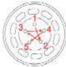
Correct tightening order for wheel bolts
