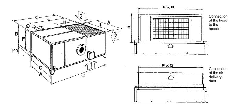
AIR INLET GRILL: on request between position 1 - 2 - 3. The head is the same of the series "AS". The order must indicate the positioning (right or left). The drawing shows the left positioning.
