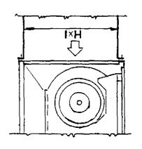
Connection of the air recovery duct
