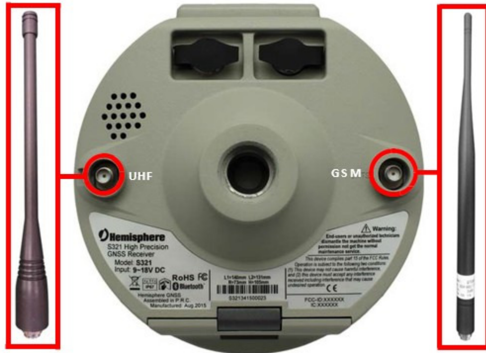
Figure 2-3: Installing UHF and GSM Antennas
