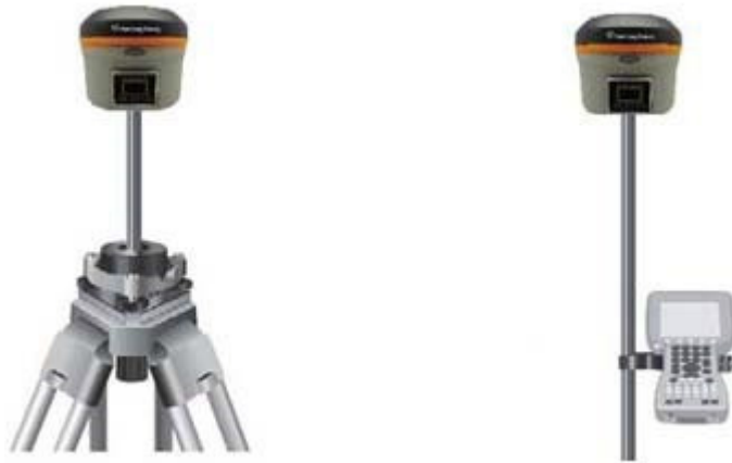
Figure 3-8: Base and Rover Setup
