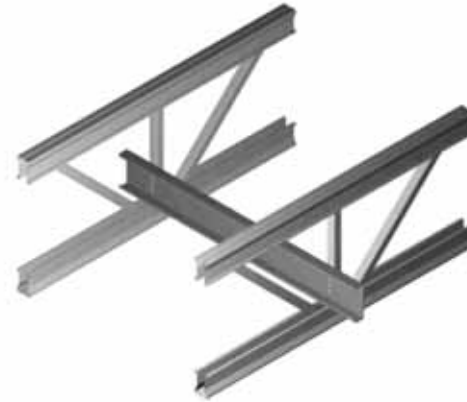
Standard strongback installed on vertical webs.
