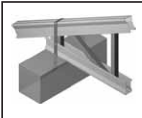
Bottom chord bearing truss to concrete bearing
