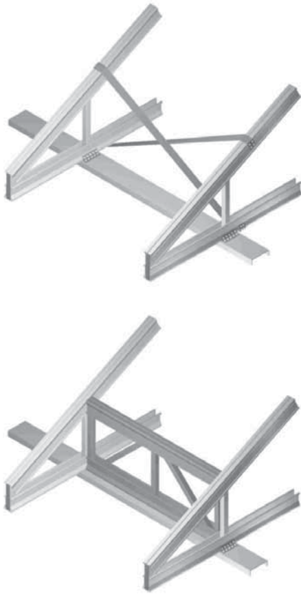
Examples of permanent bracing at truss heels, using cross-bracing (top) and trusses as blocking (bottom)
