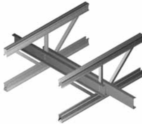
Strongback splice - overlap one truss as shown.
