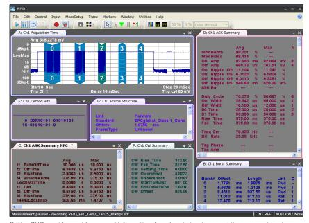
Option BHC provides a wide range of information, from burst structures and time parameters, to actual decoded bits. Additional features designed to make analyzing your signal easier include arrows on bursts to indicate direction (forward/reverse) and highlighting the current burst under analysis.
