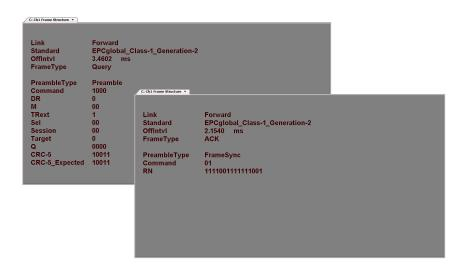
The Frame Structure table decodes the burst header data. Depending on the burst, Option BHC can decode information useful for verifying that the setup matches the demodulation parameter setup. Different standards and formats dictate which parameters are available for decoding.
