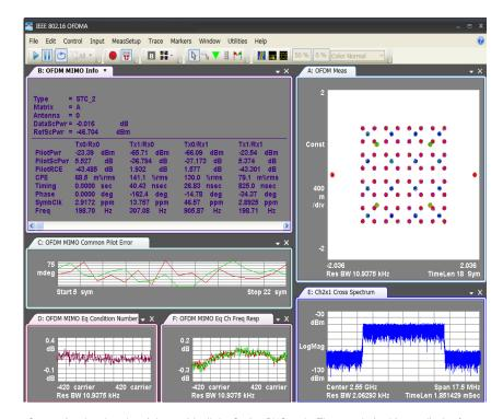
Save a signal and analyze it later with all the Option BHC tools. The cumulative history display format (Trace C), highlights signal performance over long periods. Place a marker on any point, particularly a transient outlying point, to determine its density of occurrence.
