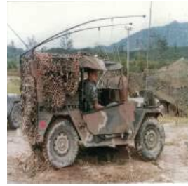
Antenna Tie Down
