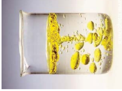
Oil and water have different polarities, so they will not form a solution.
