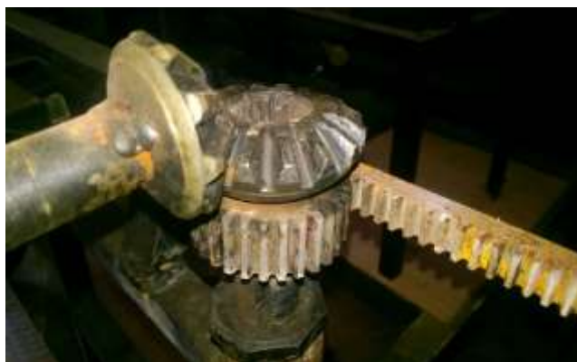
Fig. 1: Front Right Fork Gear Mechanism
