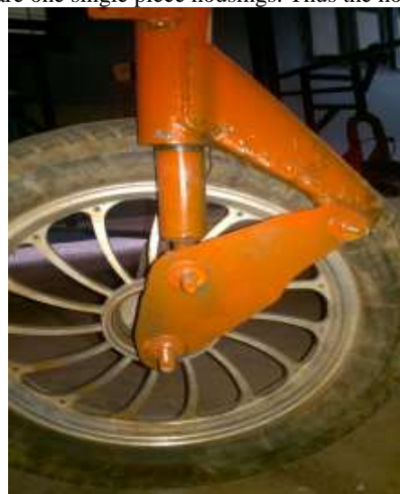
Fig. 4: Height Adjustment for Forks
