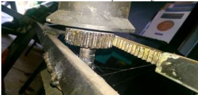
Fig. 6: Steering Rack and Pinion
