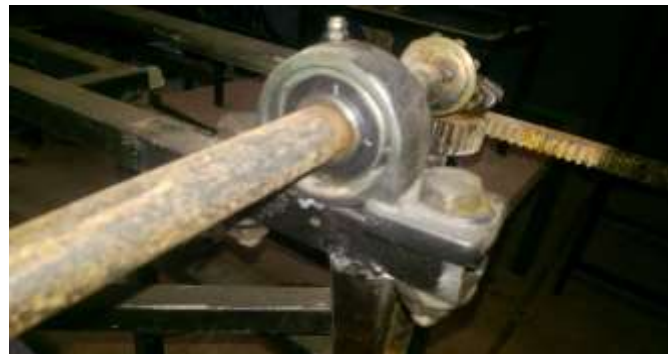
Fig. 3: Right Shaft with Plummer Block
