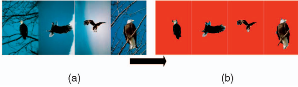
Fig. 1. Our HGM-based single-class object segmentation. (a) Inputs: A set of images each consisting of objects (foreground) of a class and different backgrounds. (b) Outputs: Regions solely containing objects of the class. The whole process is fully automatic.
