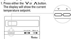
Press either the V or A button to adjust the temperature setting either up or down.
