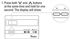
Press either the V or ∧ button to adjust the temperature differential up or down.
