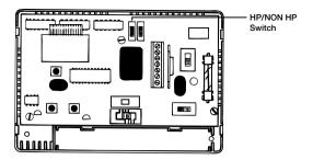
15. Install two "AA" ENERGIZER brand batteries or equivalent into battery compartment. Be sure to match positive (+) ends of batteries with positive (+) battery terminals in the battery compartment. The display will show as follows:
