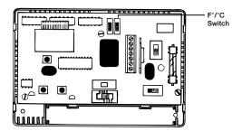
14. Put the HP/NON HP switch to either the HP for Heat Pump or NON HP for furnace applications in the proper position.
