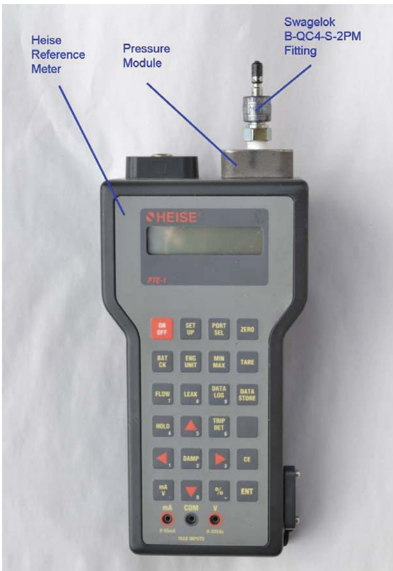
Figure 17. Heise meter with Swagelok fitting attached to pressure module.
