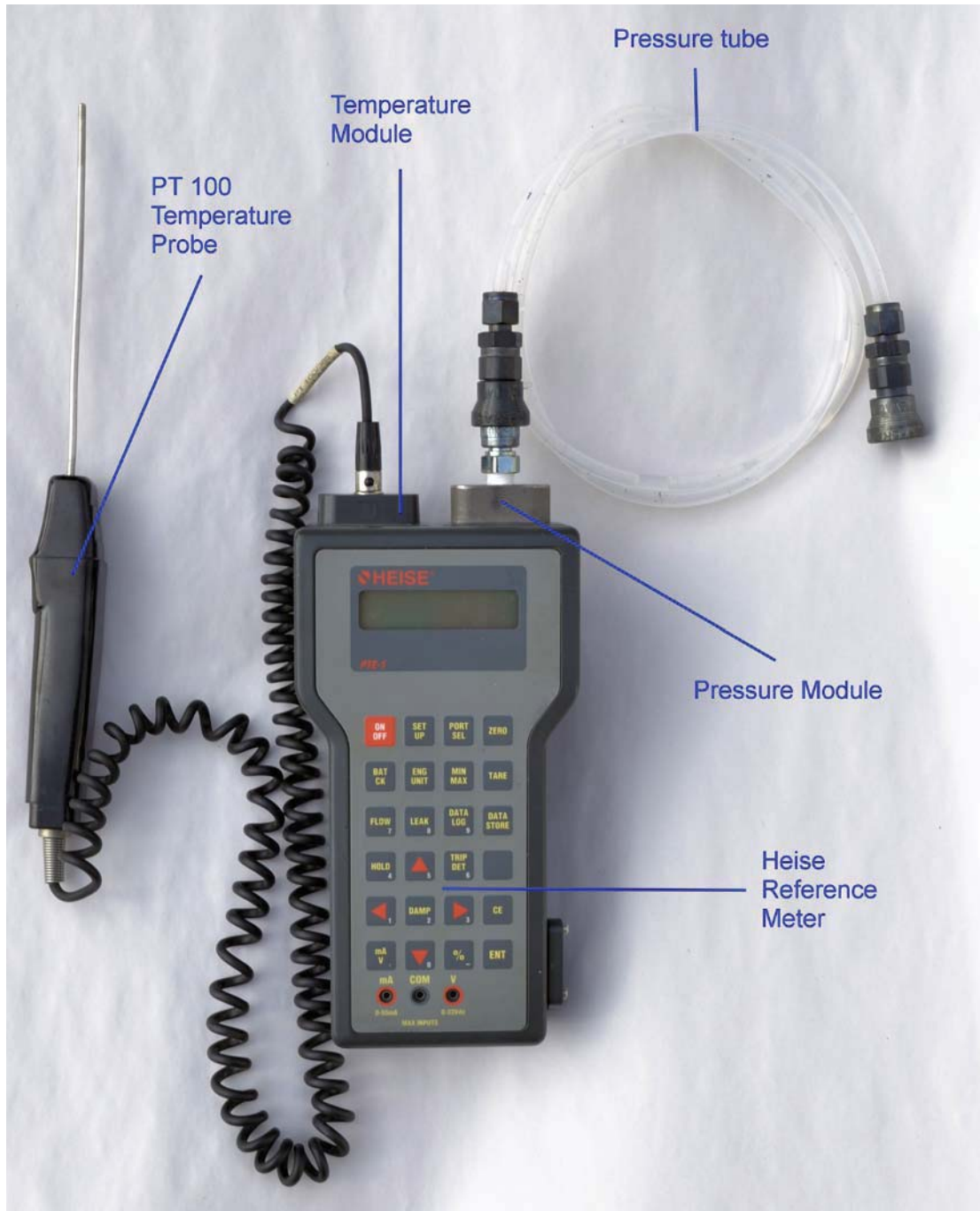
Figure 18. Heise hand held calibrator with temperature module, pressure module, PT 100 temperature probe and pressure tube.
