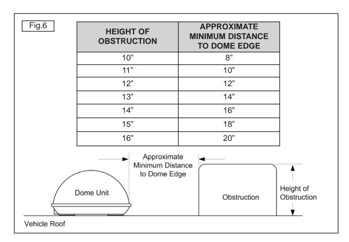
IMPORTANT! For installations on trucks with air shields, a bracket must be used for mounting the dome unit. The dome unit <u>MUST</u> be mounted to the air ride cab: <u>NEVER</u> to any structure mounted directly to the frame.
