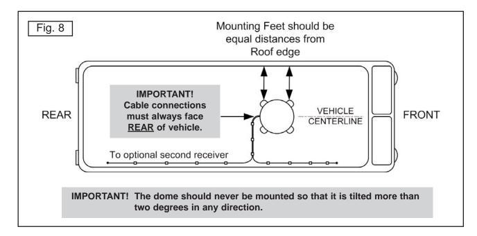
Note: The installer is responsible for determining the most appropriate fastener to secure the dome to the roof. Depending on the roof material, fasteners such as lag screws, well nuts, sheet metal screws, toggle bolts and T anchors may be used, and should always be used in combination with a roof compatible sealant.
