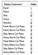
Note you can turn the visibility of different door components on or off.
