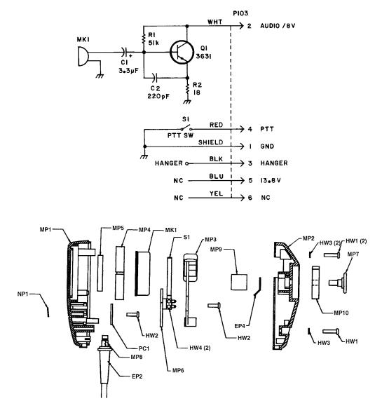
AMPLIFIED DYNAMIC MICROPHONE SCHEMATIC AND MECHANICAL PARTS Part No. 250-0740-300
