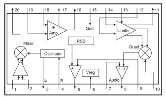
Figure 3-6 Limiter/Detector U201 Block Diagram
