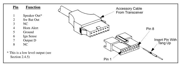
Figure 2-4 Accessory Cable Connector
