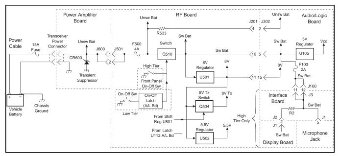
Figure 3-1 Power Distribution and Switching
