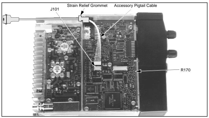
Figure 2-3 Accessory Cable Installation
