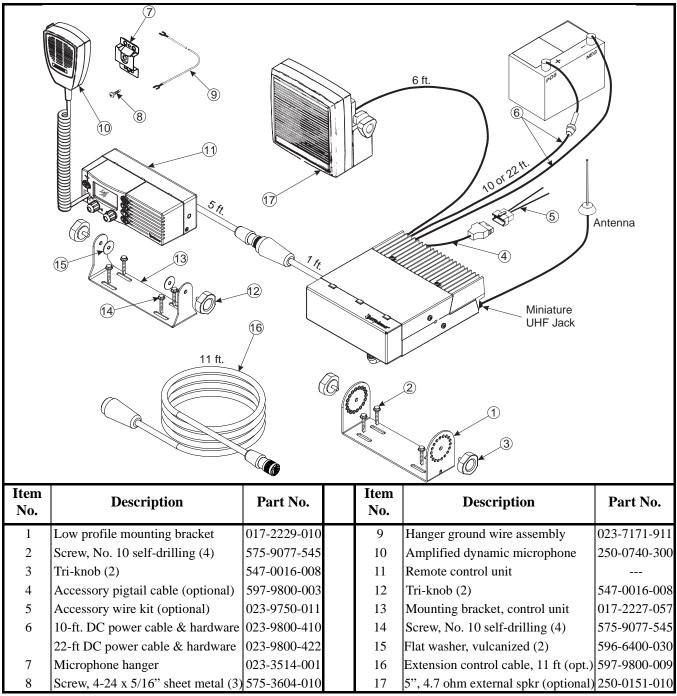
Figure 2-2 Remote Mount Installation Components
