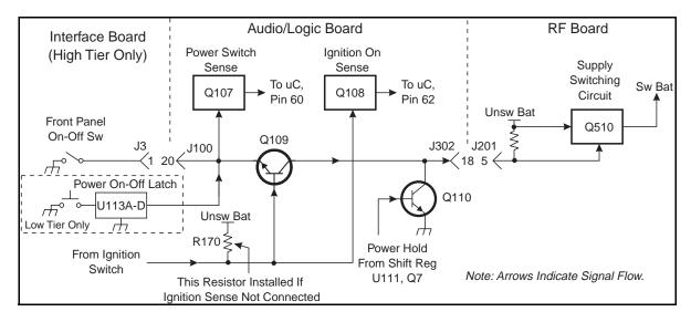
Figure 3-2 Power On-Off Control Circuit
