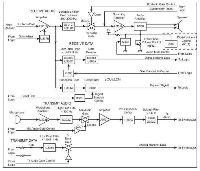
Figure 3-3 Audio and Data Processing Circuitry Block Diagram
