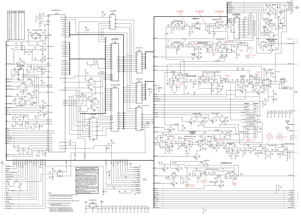
AUDIO/LOGIC BOARD SCHEMATIC
