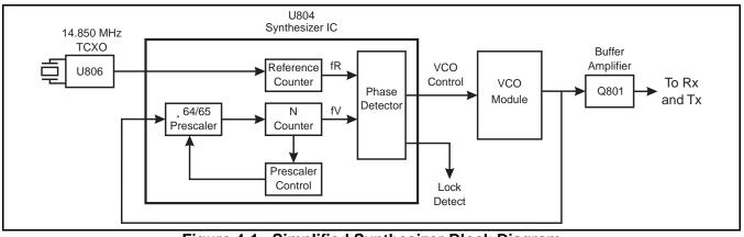
Figure 4-1 Simplified Synthesizer Block Diagram
