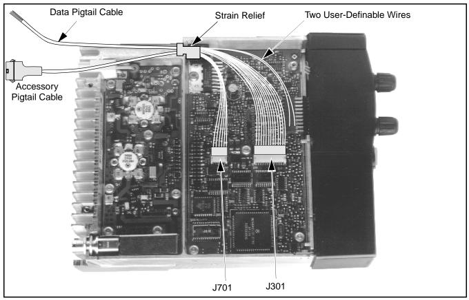
Figure 2-6 Data Cable Installation (-001 Cable Shown)
