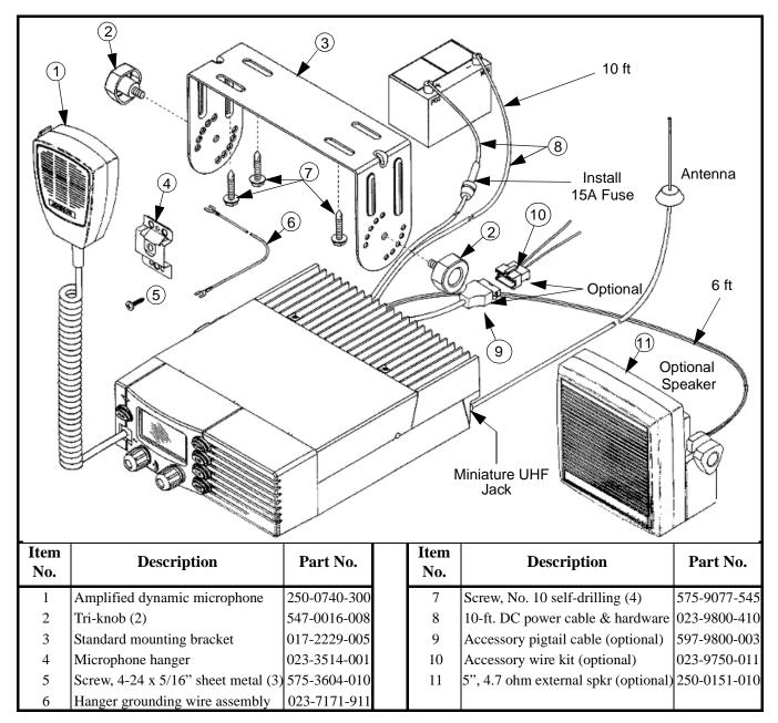
Figure 2-1 Front Mount Installation Components
