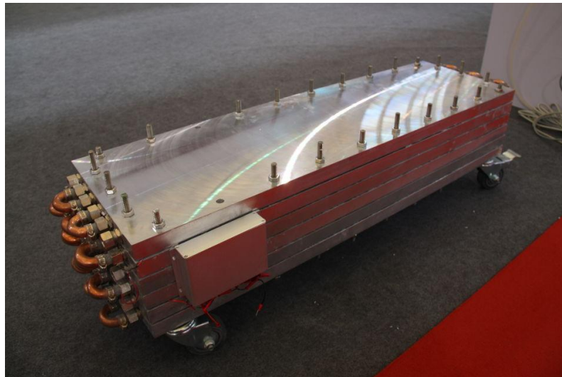
Figure 12: The 1 KW thermoelectric generator for low-temperature geothermal resources
