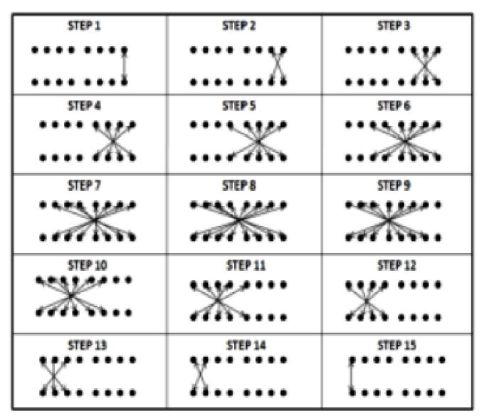
Fig.8-bit binary multiplication using Urdhva Tiryakbhyam Sutra
