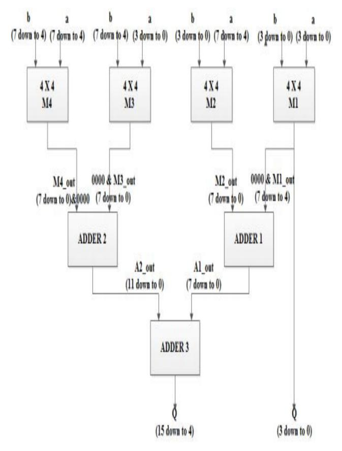
Fig.: Hardware realization of 8 x 8 multiplier
