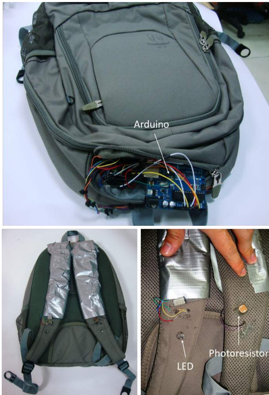
Figure 4.19: The internals of the Intelligent Straps bag.
