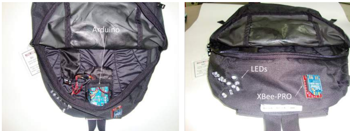
Figure 4.17: The electronic components in the Maxwell Bag prototype
