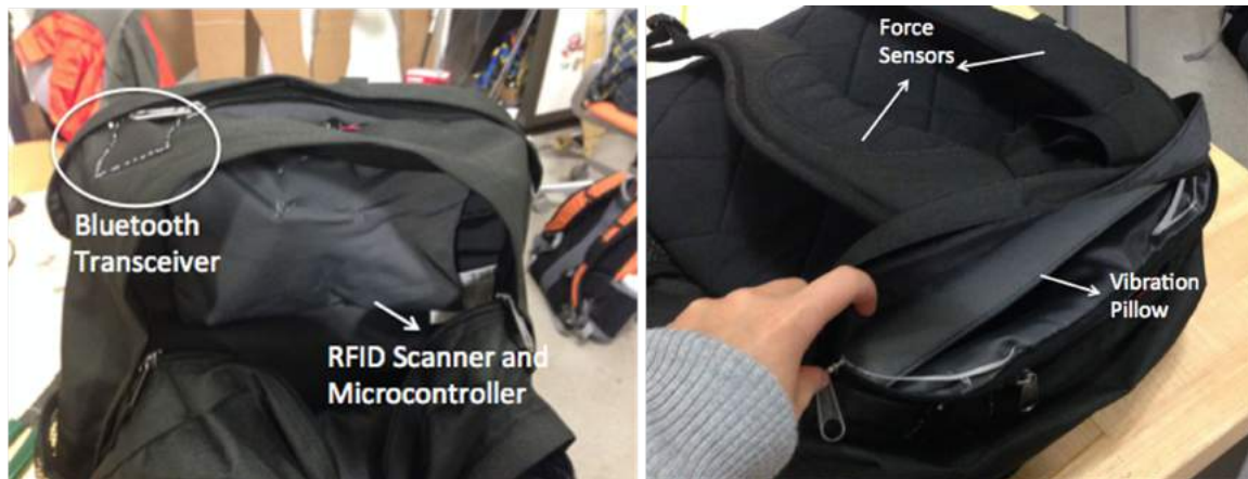
Figure 5.2: The ForgetMeNot bag with electronics hidden from user
