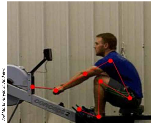
Figure 1: Illustration of a biomechanical model created from a digitized frame of the rowing video.
