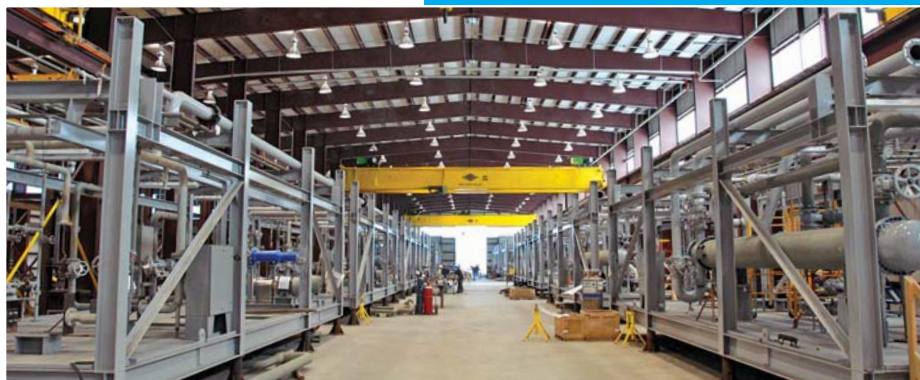
Existing 6,000 barrel-a-day Refinery- Modular Unit in Texas ready for immediate shipment and assembly
