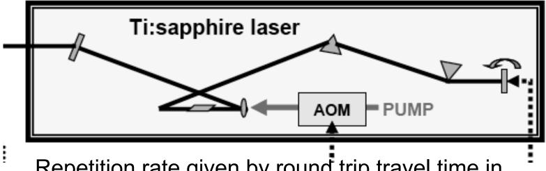
Repetition rate given by round trip travel time in cavity. Modulated by piezo adjustment of cavity mirror.
