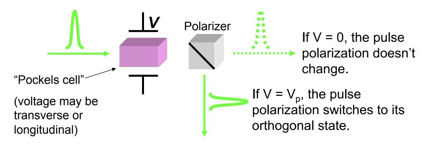
Abruptly switching a Pockels cell allows us to switch a pulse into or out of a laser.
