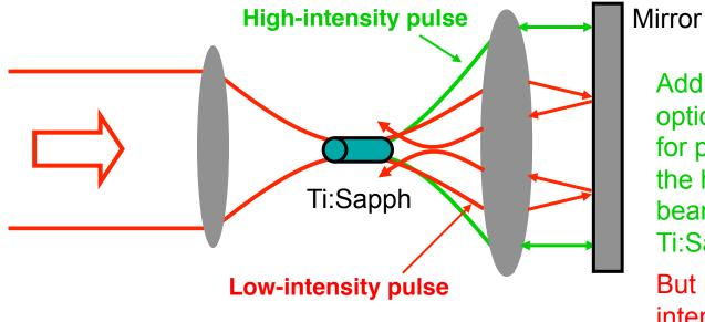
Additional focusing optics can arrange for perfect overlap of the high-intensity beam back in the Ti:Sapphire crystal.
