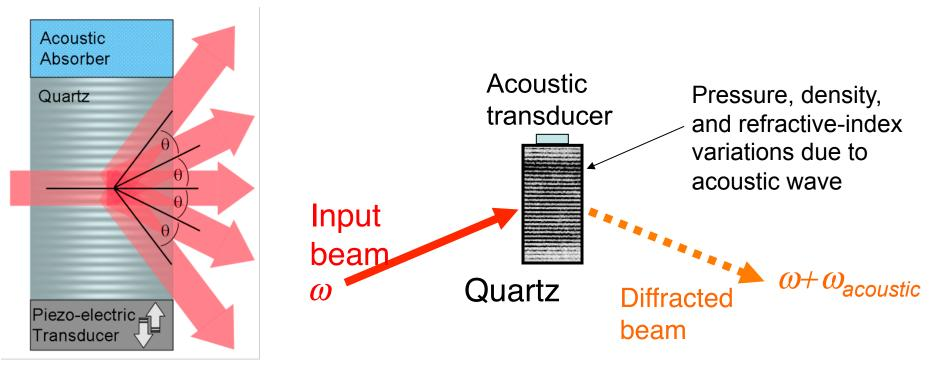
Acousto-optics works because acoustic waves have about the same wavelengths as (visible) light waves. Such diffraction can be quite strong: ~70%. Acousto-optics is the basis of useful devices.
