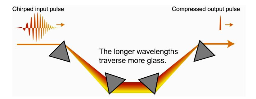
It's routine to stretch and then compress ultrashort pulses by factors of >1000
