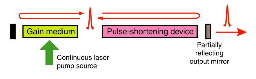
Pulse-shortening devices include: Saturable absorbers Phase modulators Dispersion compensators Optical-Kerr media
