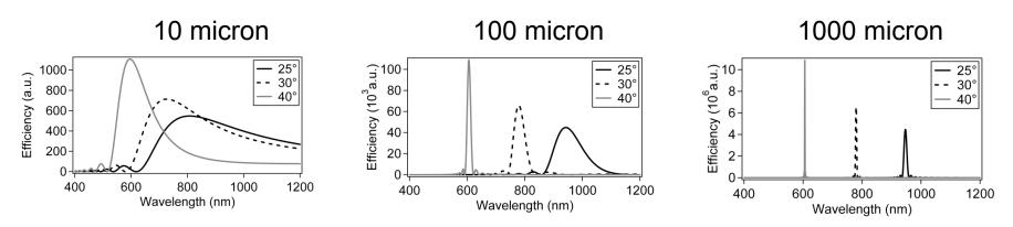
Note the huge differences in phase-matching bandwidth and efficiency with crystal thickness.
