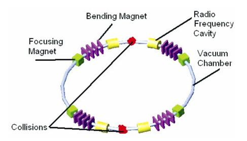
In an accelerator, focusing magnets and bending magnets guide the beam of particles around a ring. (Only a few of the bending magnets are shown here). High frequency microwave (*RF*) cavities accelerate the beams as they pass through.
