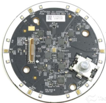
Figure 12: Microphone array on Amazon Echo™. (from [202])
