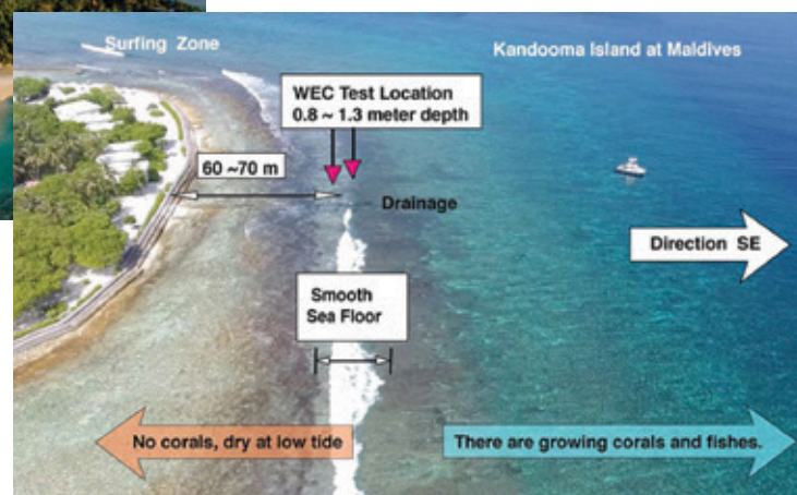
■ Okinawa Institute of Science and Technology Wave Energy Project. Two wave energy converter units are being tested at the southeast side of Kandooma island (South Male-atoll) (photos by Ministry of Environment).
