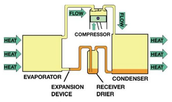
Condensers on both TXV and Orifice Tube Systems are designed to have 10 to 20 degrees Fahrenheit of Sub-Cooling.
