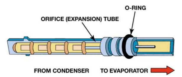
An Orifice Tube System most commonly runs a flooded evaporator and has very low Superheat. They will have 0 to 4 degrees Fahrenheit of Superheat.
