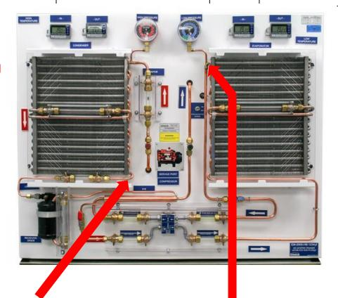
TYPICAL H-BLOCK (TXV) SYSTEM WITH IHX (INTERNAL HEAT EXCHANGER
