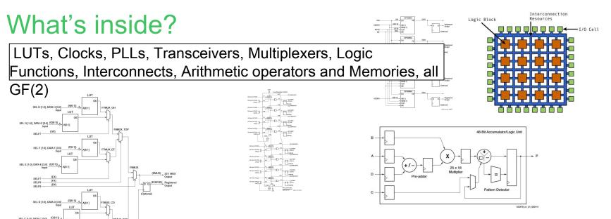
Hundreds of thousands of these programmable logic block widgets! They can be interconnected to create logic that can accomplish just about anything. A major part of the device programming involves place and route (the tools do this for you) which is how all the interconnects are setup to put it all together.
