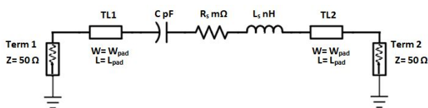
Fig. 1. Capacitor equivalent model.
