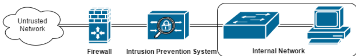
Figure 2 - Example of an inline IPS implementation
