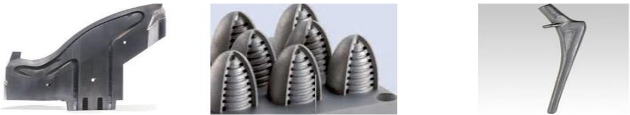
Fig. 7: SLM steel insert with conformal cooling [26], SLM tool inserts with conformal spiral cooling [27], LENS titanium hip stem[23].
