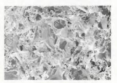
Fig. 17 — Metallographic cross-sections and SEM fractograph of multiphase BNi-2 lap shear failure. Note brittle fracture surface
