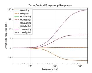
Figure 2: Tone control frequency response at various values of the Treble parameter, comparing the responses of the analog filter with the digital model.
