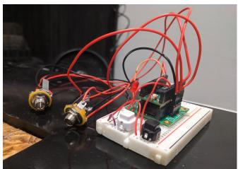
Figure 12: Teensy microcontroller implementation.
