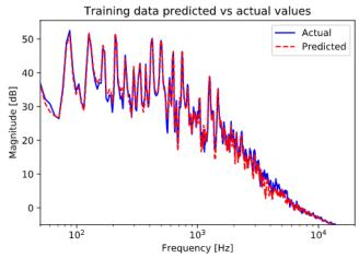
Figure 7: Comparison of predicted output of the model against reference output shown in the time domain (above) and frequency domain (below). The frequency domain plot uses frequency band smoothing using 1/24 octave bands for improved clarity.
