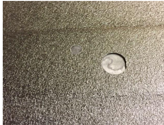
Flat bottom holes *Significant delamination
