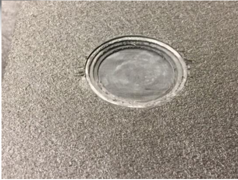
Concentric flat bottom holes *Impact damage
