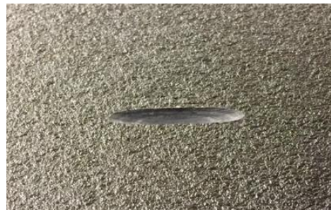
Grinder Disk Groove *Gouge or deep scratch
