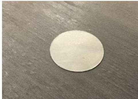
Grafoil® insert *Tight delamination
