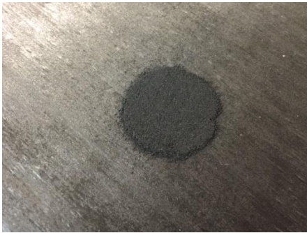
Carbospheres *Localized porosity
