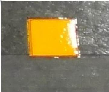
Pillow insert *Delamination
