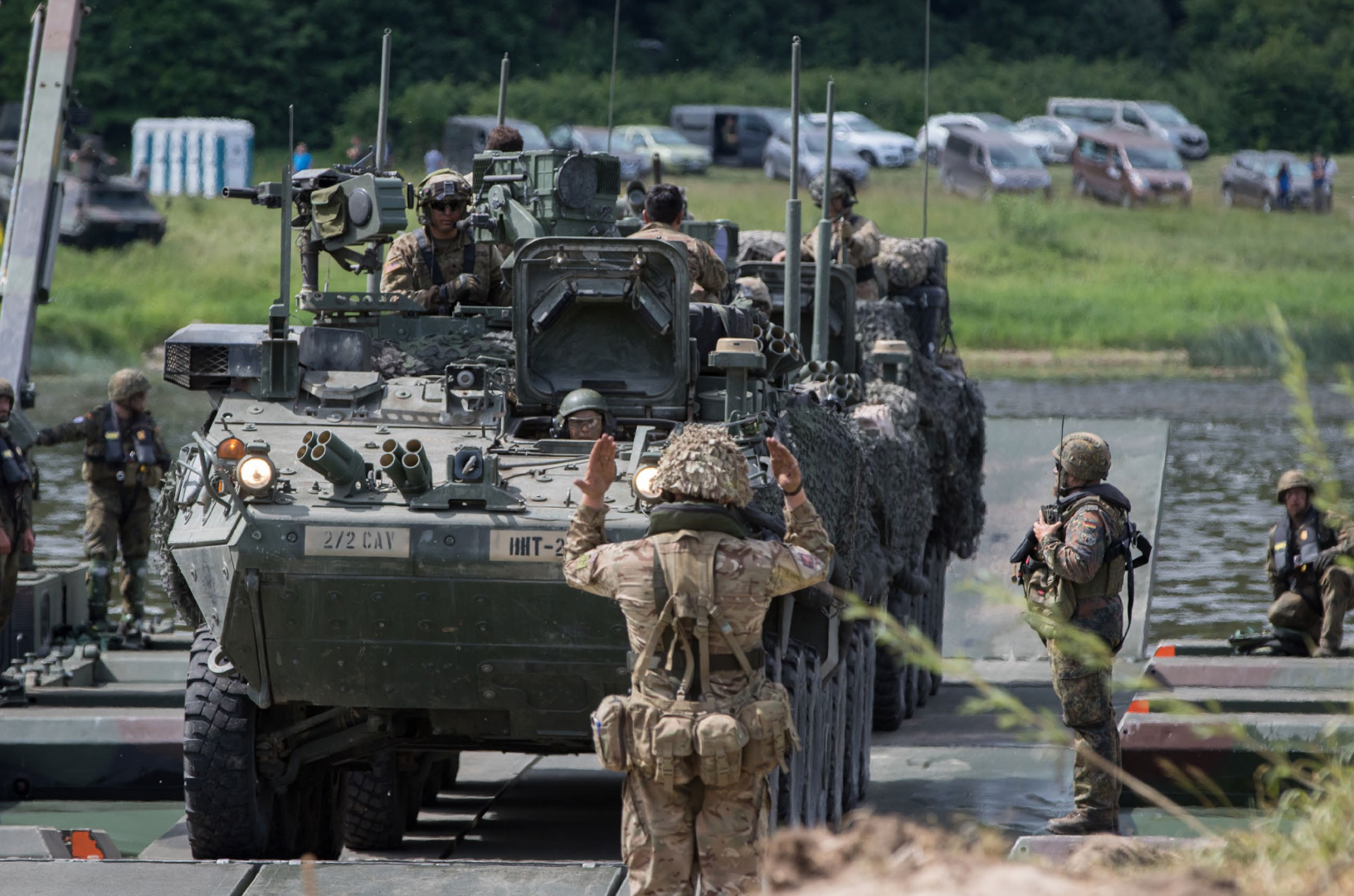
A British soldier directs Stryker vehicles from 2nd Cavalry Regiment as they cross the Nemen River in Lithuania using an Amphibious Rig Bridge. Taken during Exercise Saber Strike in June 2018. Source link: Wikimedia Commons/Spc. Andrew McNeil, US Army https://commons.wikimedia.org/wiki/File:Cavalry_Crosses_River,_Continues_Road_March_180613-A-OL598-318.jpg
