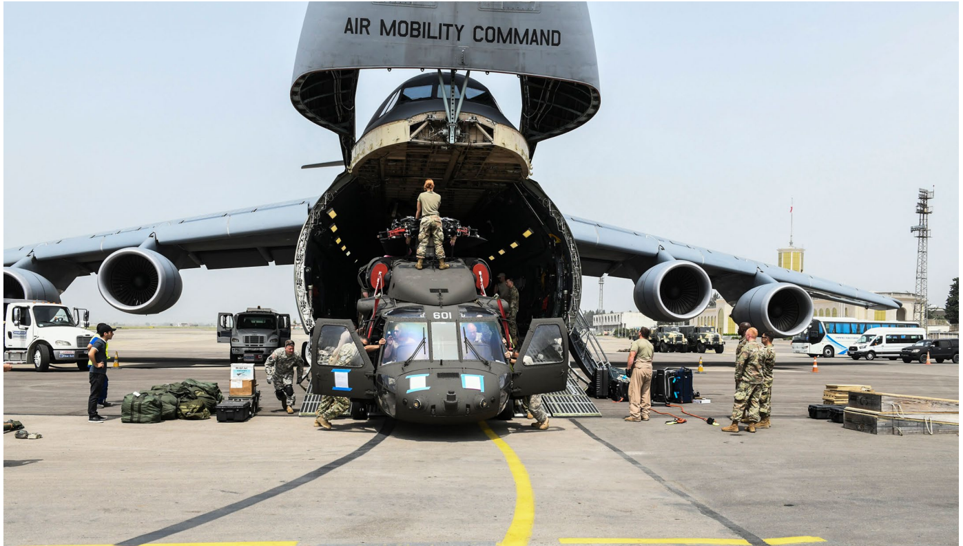
Georgia State Air National Guard personnel unloading a UH-60 Black Hawk helicopter from a C-5 Galaxy strategic airlifter as part of Exercise Noble Partner 2018 in Georgia. Source link: US Army Europe Flickr https://www.flickr.com/photos/usarmyeurope_images/42972584814/in/album-72157699139027644/
