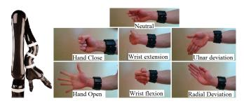
Fig. 1. The 7 gestures considered in this work. The Myo armband (right) is connected through bluetooth to the laptop. The computer, after data analysis, transfer the command to JACO (left) in real-time via a USB connection.
