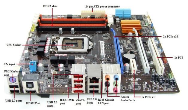
**Motherboard Components:** A typical Micro ATX motherboard with constituent components is given below:
