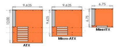
Further, Mini ITX is limited to one PCI-e slot, and up to 2 memory slots. For most PC applications, Mini-ITX is sufficient unless you want to go for more PCI-e slots or do heavy gaming (display-intensive).
