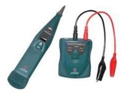
**4. Cable Tester :** A cable tester is used to verify that all of the intended connections exist and that there are no unintended connections in the cable being tested. When an intended connection is missing it is said to be "open". When an unintended connection exists it is said to be a "short" (as in short circuit). If a connection "goes to the wrong place" it is said to be "miswired" (the connection has two faults: it is open to the correct contact and shorted to an incorrect contact).
