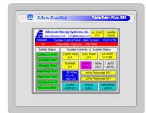
Optional EOI for Allen-Bradley PLC: 6-inch PanelView-Plus display with first-out monitor (Alarm History) and graphic TrendLine recording. Applications developed for this EOI can also run on a PC with FactoryTalk View ME Station license (for remote monitoring).
