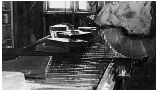
Circular saw cutting slate. Photograph by Neil Rappaport. (Slate Valley Museum)
