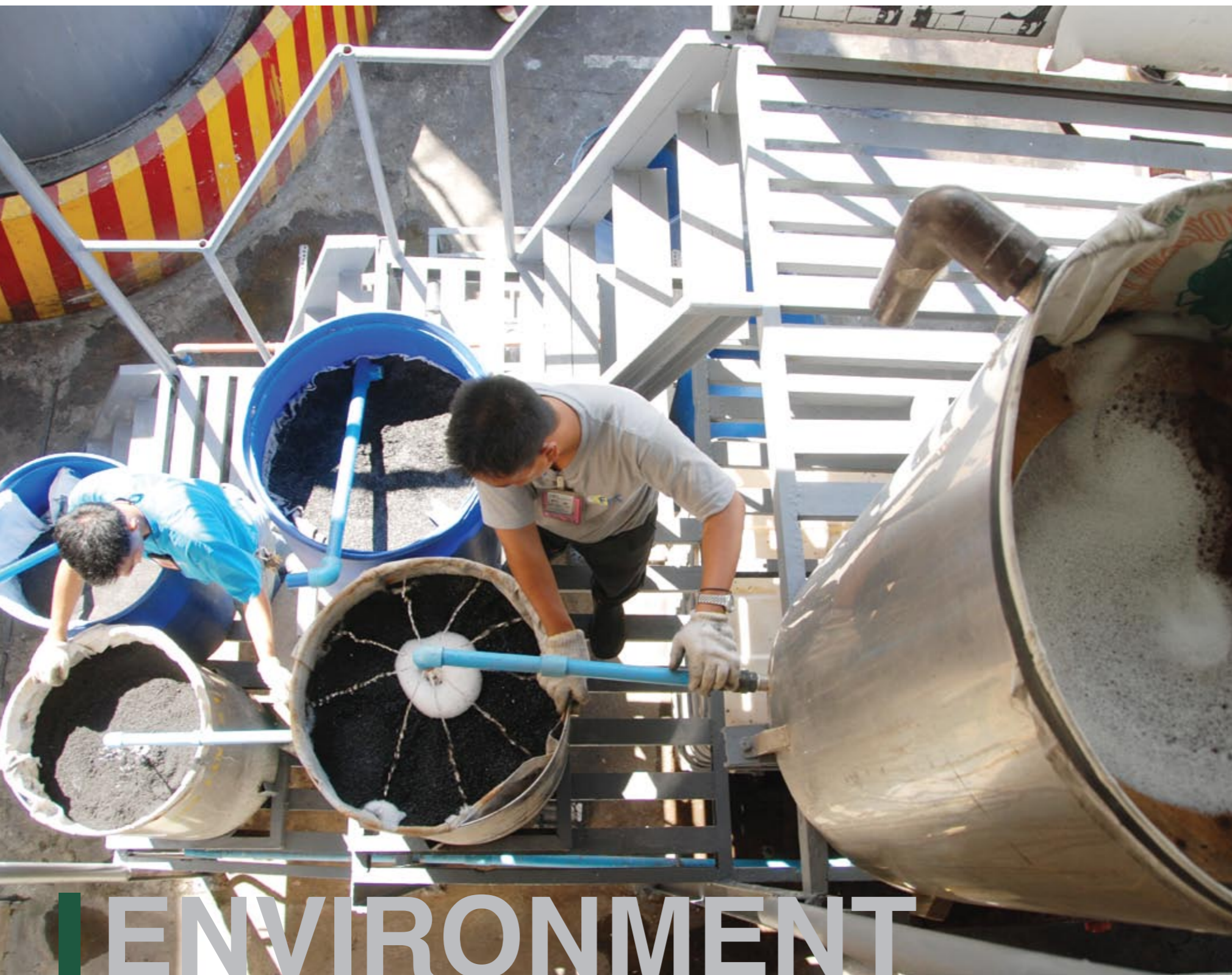
Nestlé business partner Fortune Packaging Corporation has developed a low-cost wastewater treatment plant using scrap materials
