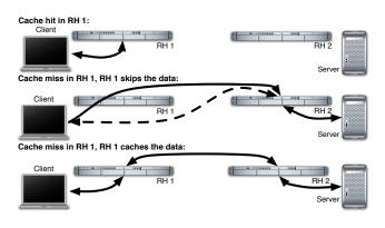
Figure 5: Three cases of processing a FIND packet when caching is supported: serve from the cache, skip (merely forward the FIND), and cache. RH 2 is a middlebox for all traffic.
